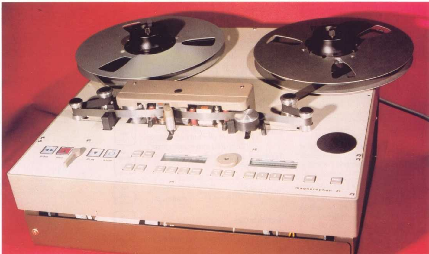
Fig. 1 Magnetophon 21-1/2" as a table model - A-wind shown
